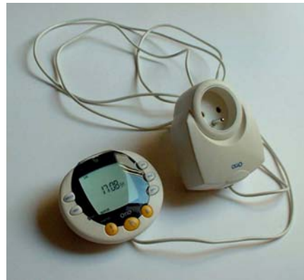
An electronic timer unit to control the mains electricity supply to the power supply unit (battery charger or other) with digital display and setting buttons on an extension lead.
