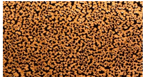
Below – magnified photograph of copper plate with reticulated black ink ground after salt tint has been dissolved
