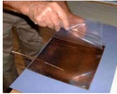
Above - self adhesive plastic tape laid over back of plate to fix copper contact strips.
