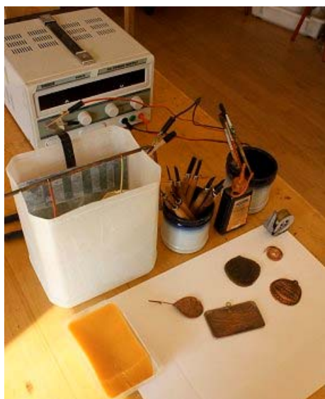
Equipment and tools for casting small copper objects – 10 amp power supply, small tank with bar to hang moulds, wax, modelling tools, graphite powder, copper and brass wire, small wax moulds ready for modelling
