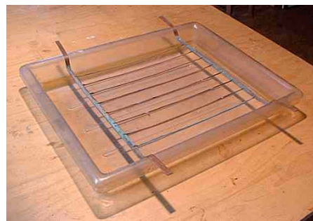
Copper backplate contact with copper strip bent up to project out of electrolyte - strip protected by strong varnish.
